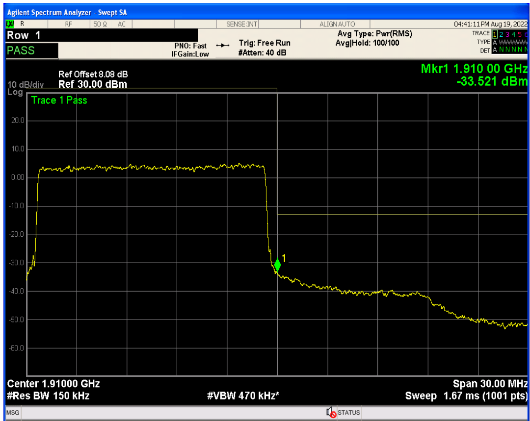
Band2 QPSK BW=15MHz Channel=19125 RB Size=1 Position=#Max
