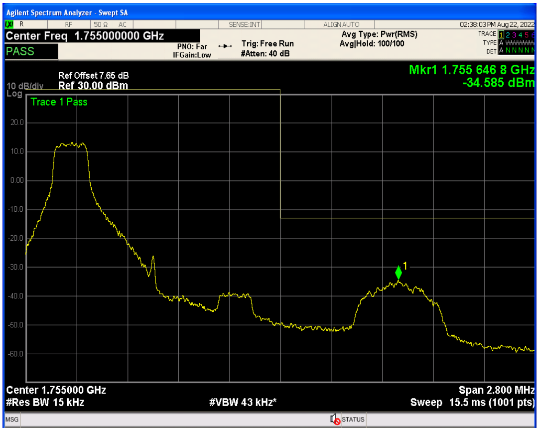
Band4 QAM16 BW=1.4MHz Channel=20393 RB Size=1 Position=#Max
