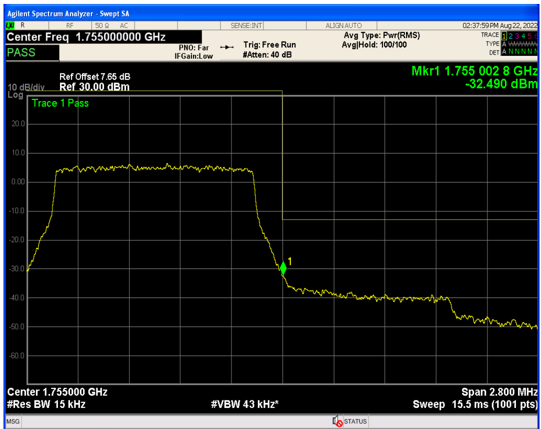
Band4 QAM16 BW=1.4MHz Channel=20393 RB Size=1 Position=#0
