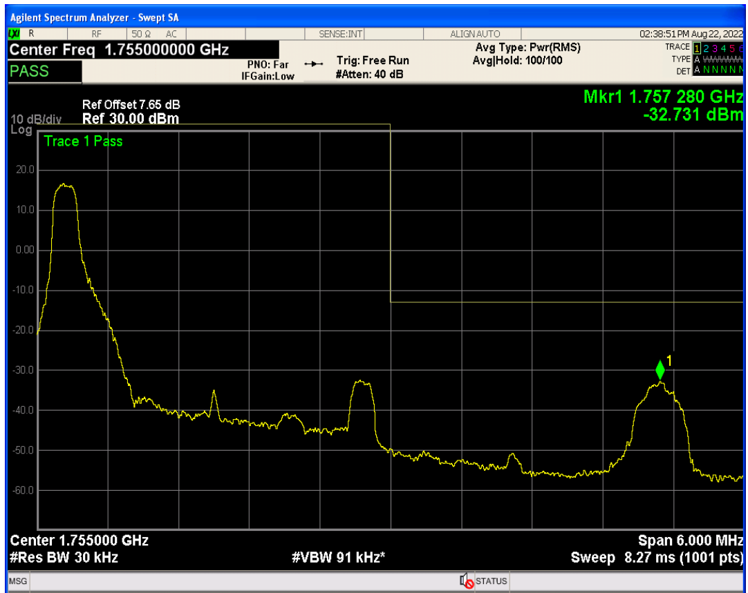
Band4 QAM16 BW=3MHz Channel=19965 RB Size=15 Position=#0
