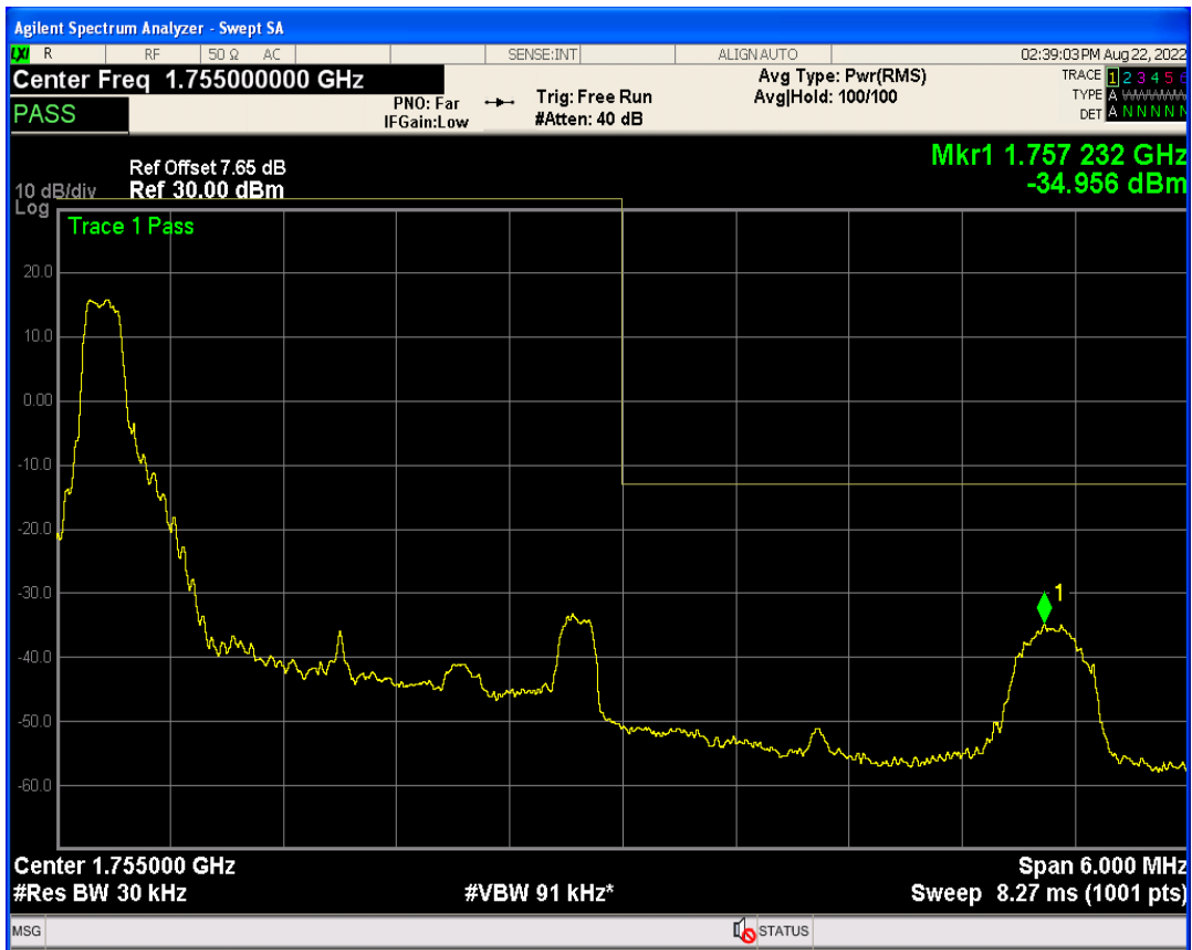
Band4 QAM16 BW=3MHz Channel=20385 RB Size=1 Position=#Max
