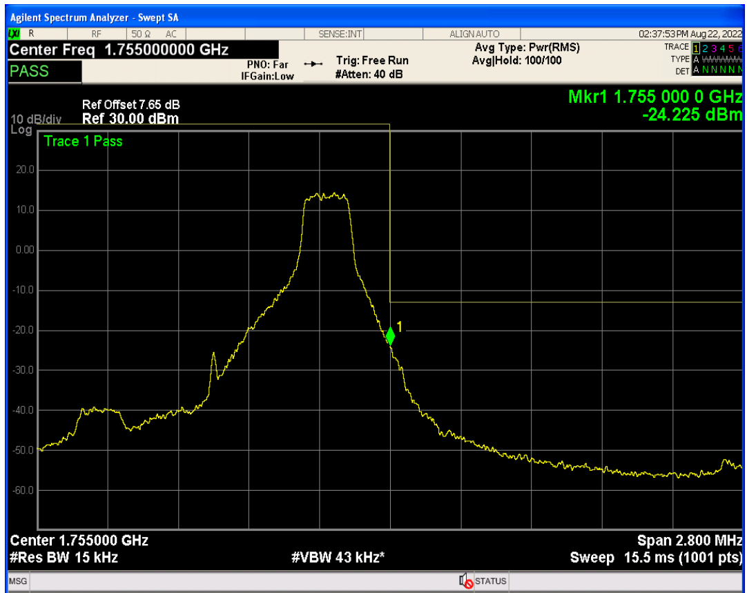
Band4 QPSK BW=1.4MHz Channel=20393 RB Size=6 Position=#0
