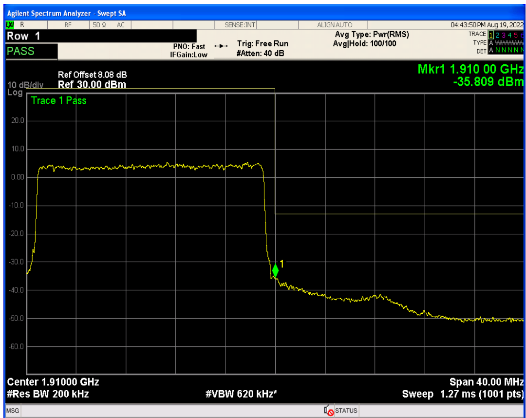
Band2 QAM16 BW=20MHz Channel=19100 RB Size=1 Position=#Max
