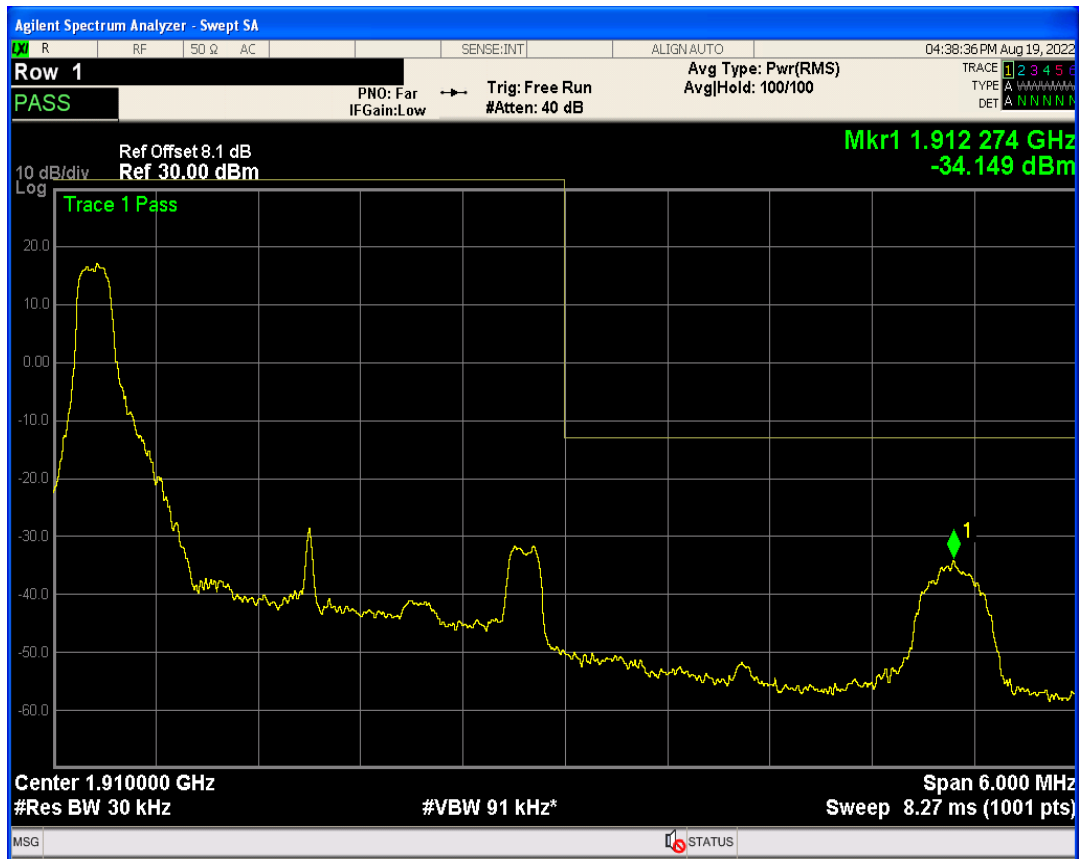
Band2 QAM16 BW=3MHz Channel=18615 RB Size=15 Position=#0
