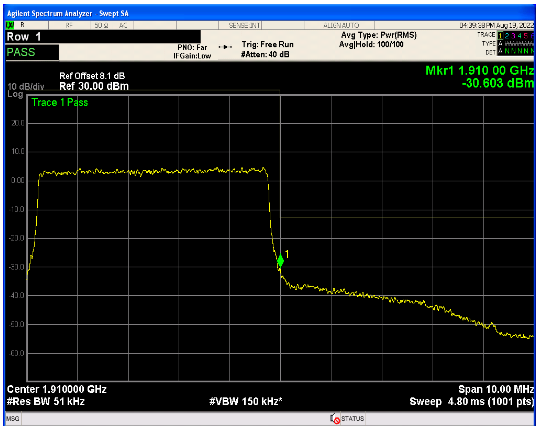
Band2 QAM16 BW=5MHz Channel=19175 RB Size=1 Position=#Max
