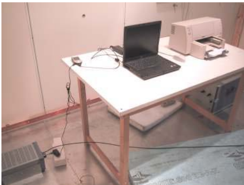
Picture 2: Conducted emission test setup.
