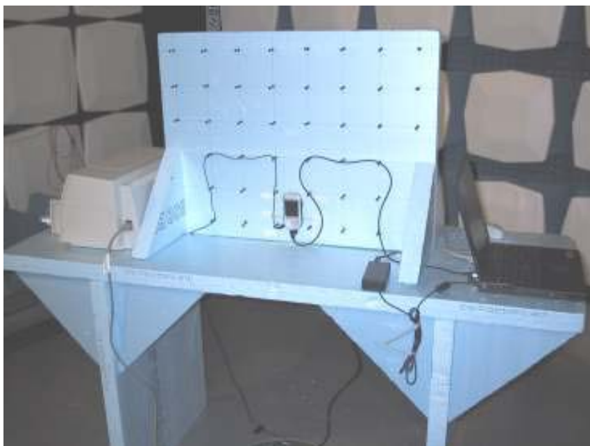
Picture 1: Radiated emission test setup.
