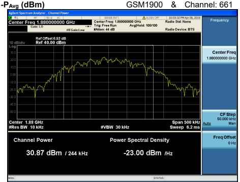
PAPR (dB) = P<sub>Pk</sub> (dBm) - P<sub>Avg</sub> (dBm) = 30.93 dBm - 30.87 dBm = 0.06 dB
