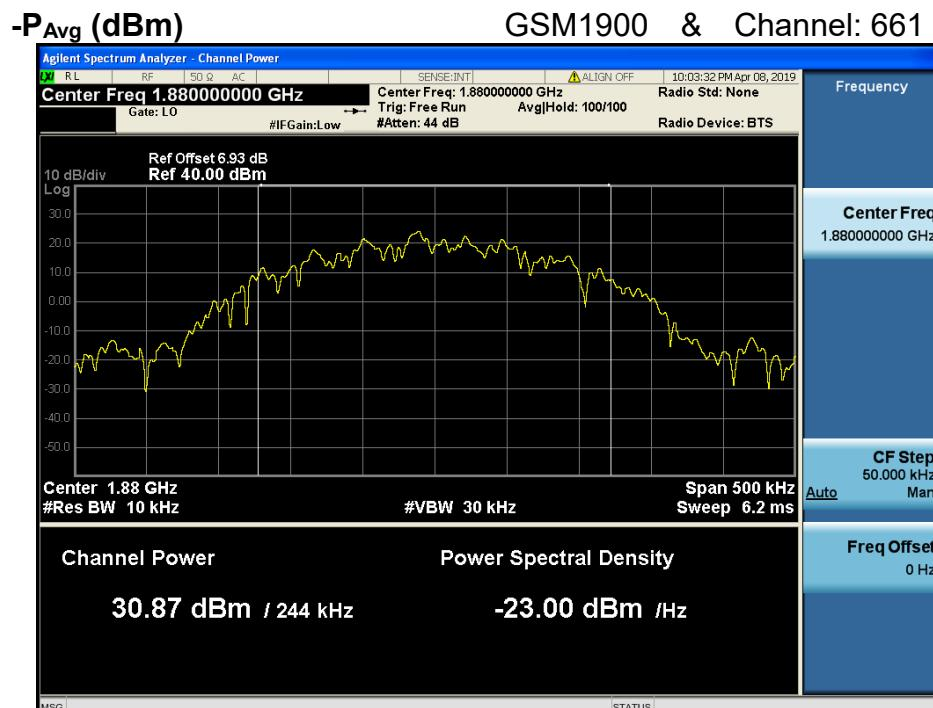
$$\text{PAPR (dB)} = \text{P}_{\text{Pk}} (\text{dBm}) - \text{P}_{\text{Avg}} (\text{dBm}) = 30.93 \text{ dBm} - 30.87 \text{ dBm} = 0.06 \text{ dB}$$
