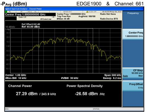
$PAPR (dB) = P_{Pk} (dBm) - P_{Avg} (dBm) = 30.93 dBm - 27.29 dBm = 3.64 dB$
