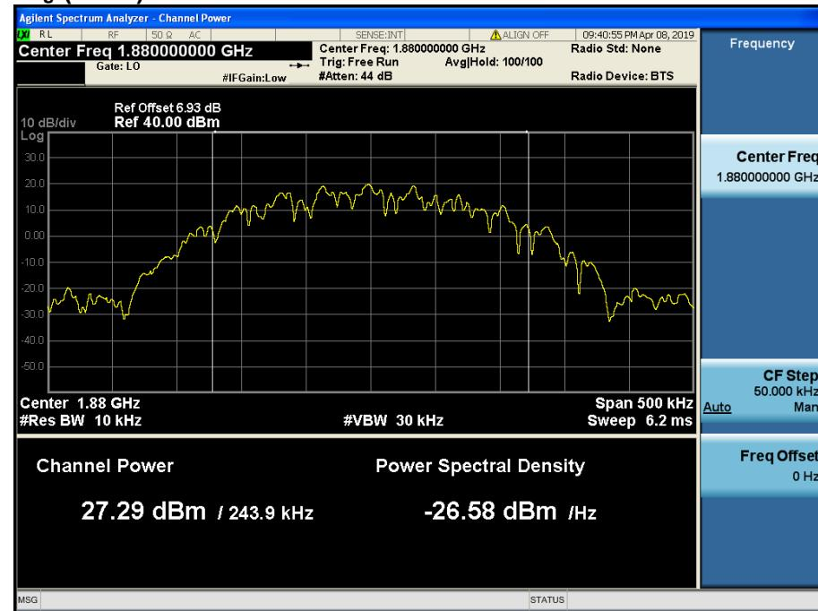
$$\text{PAPR (dB)} = \text{P}_{\text{Pk}} (\text{dBm}) - \text{P}_{\text{Avg}} (\text{dBm}) = 30.93 \text{ dBm} - 27.29 \text{ dBm} = 3.64 \text{ dB}$$
