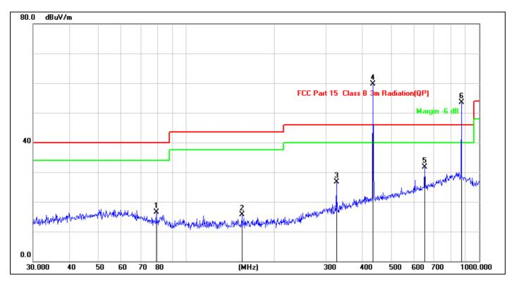
Site: LAB Antenna::Horizonta **Temperature(C):26(C) Humidity(%):60%** Limit: FCC Part 15 C 3m Radiation **Test Time:** 2023/03/02 9:07:21 **EUT: RF Remote Controller** M/N.: DC 3V AS-2301 **Power Rating:** Mode: TX**Test Engineer: Sunshine** Note:
