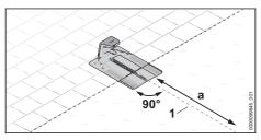
The docking station is partly in a navigable area and partly in the mowing area and the guide wire (1) can be routed in a straight line from the docking station into the mowing area over a length a = 6.6 ft. (2 m).
