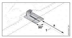
The docking station is partly in a bed and partly in the mowing area and the guide wire (1) can be routed in a straight line from the docking station into the mowing area over a length a = 6.6 ft. (2 m).
