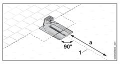
The docking station is at the edge of the mowing area. The adjacent area is navigable and the guide wire (1) can be routed in a straight line from the docking station into the mowing area over a length a = 6.6 ft. (2 m).
