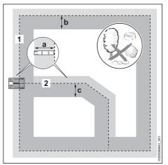
Make sure that the mowing area along the perimeter wire and the guide wire is flat and clear of obstacles as far as possible along the following widths:
