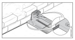
If the docking station has been positioned directly against a wall, it is also possible to install the connecting cord under the base plate. The connecting cord can be routed out of the base plate to the left or right.
