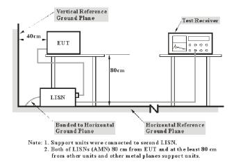
The setup of EUT is according with per ANSI C63.10-2013 measurement procedure. The specification used was with the FCC Part 15.207 and the RSS-Gen limits.
