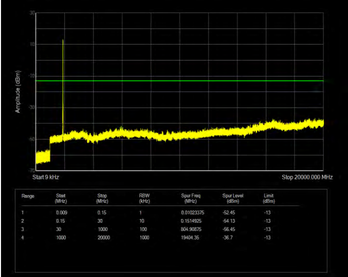
Band2 16QAM BW=10MHz Channel=19150 RB Size=50 Position=#0
