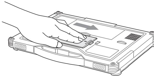
Step 3. Lift the battery out of the battery bay.
