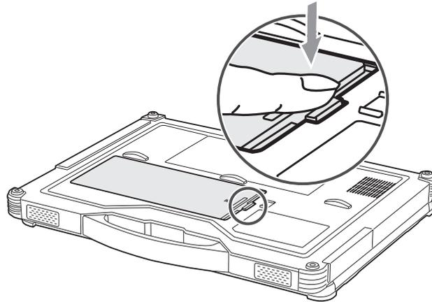
Step 2. Slide the battery towards the latch.
