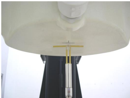
Fig 7.2 Photo of Dipole Setup
