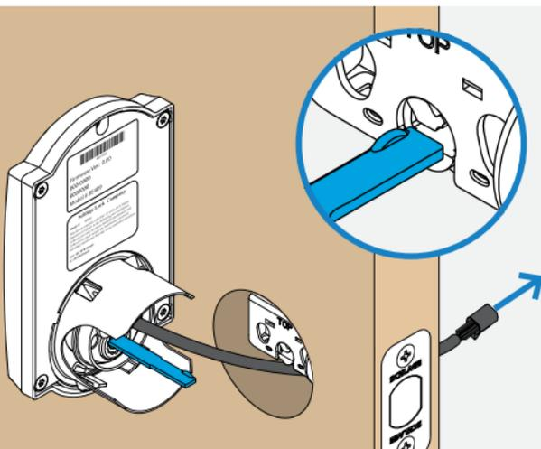
The bump on the tailpiece aligns with the slot in the bolt.
