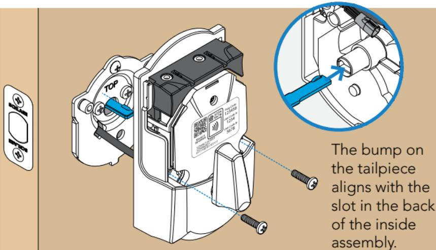
The bump on the tailpiece aligns with the slot in the back of the inside assembly.
