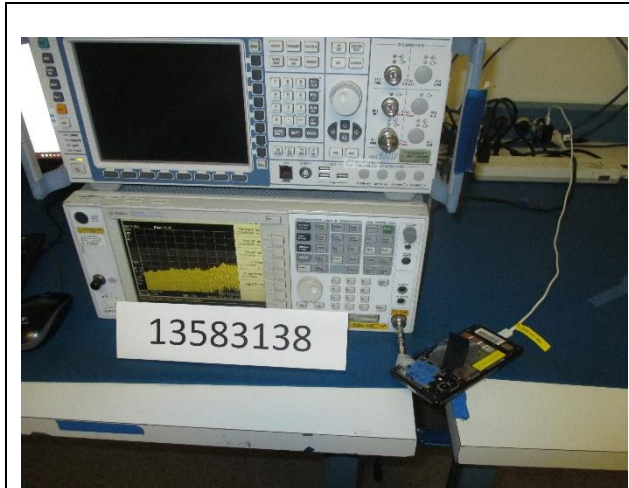
RF ANTENNA PORT CONDUCTED
