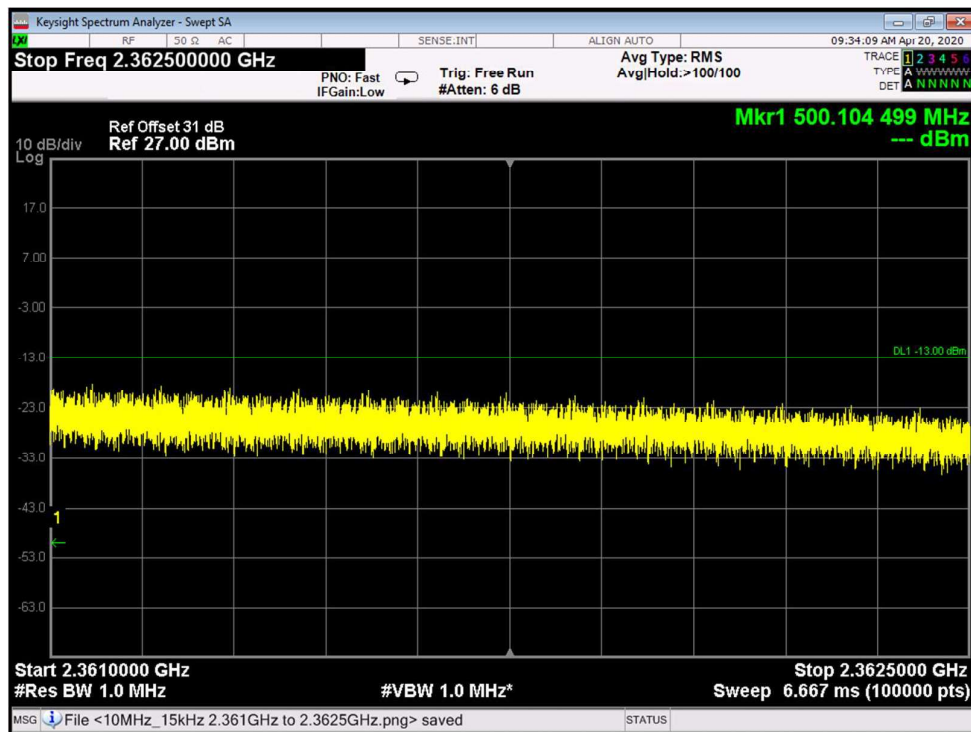
Figure 48: Spurious Emissions at Antenna Terminal 16QAM, 2355.0MHz, B.W. 10MHz, Sub Carrier 30kHz
