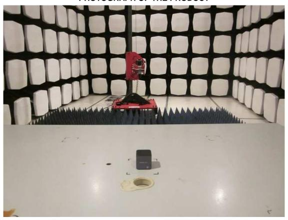
**MEASUREMENT OF CONDUCTED EMISSION TEST SET UP**
