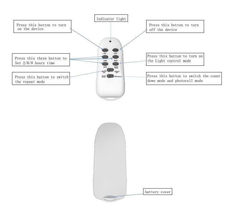
This is a transmitter used for control the device, the device maybe a light, fixed camera, home appliances and so on. The receiver usually connected the control switch which can control the device on and off.
