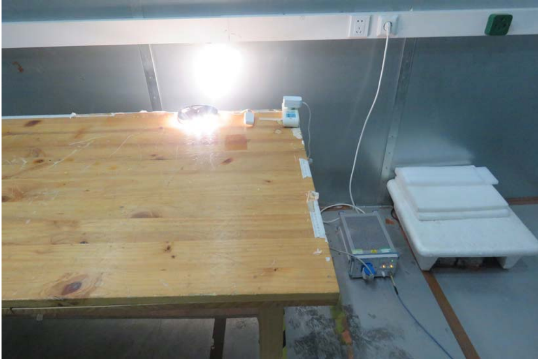
Picture 3 Conducted Emission Test Setup
