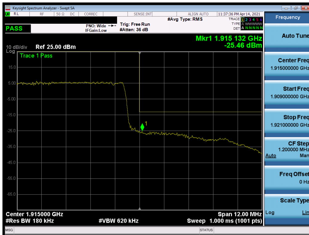
Plot 7-123. Upper Band Edge Plot (LTE Band 25 - 15MHz QPSK – Full RB)
