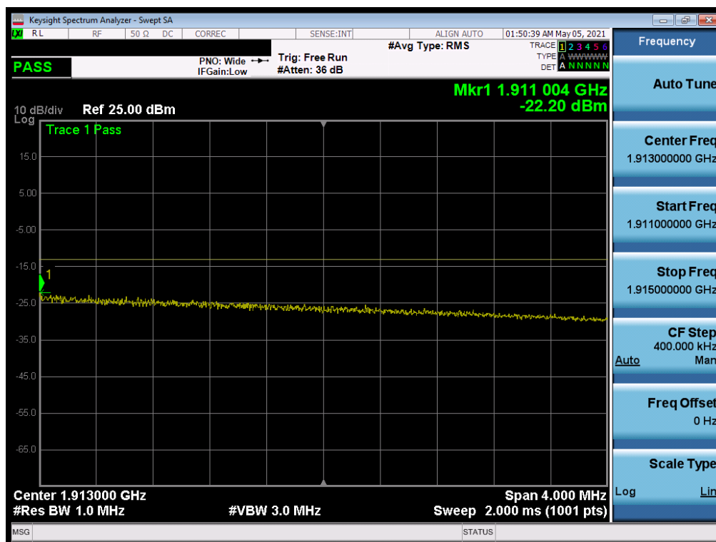
Plot 7-200. Extended Upper Band Edge Plot (NR Band n2 – 20MHz QPSK – Full RB)
