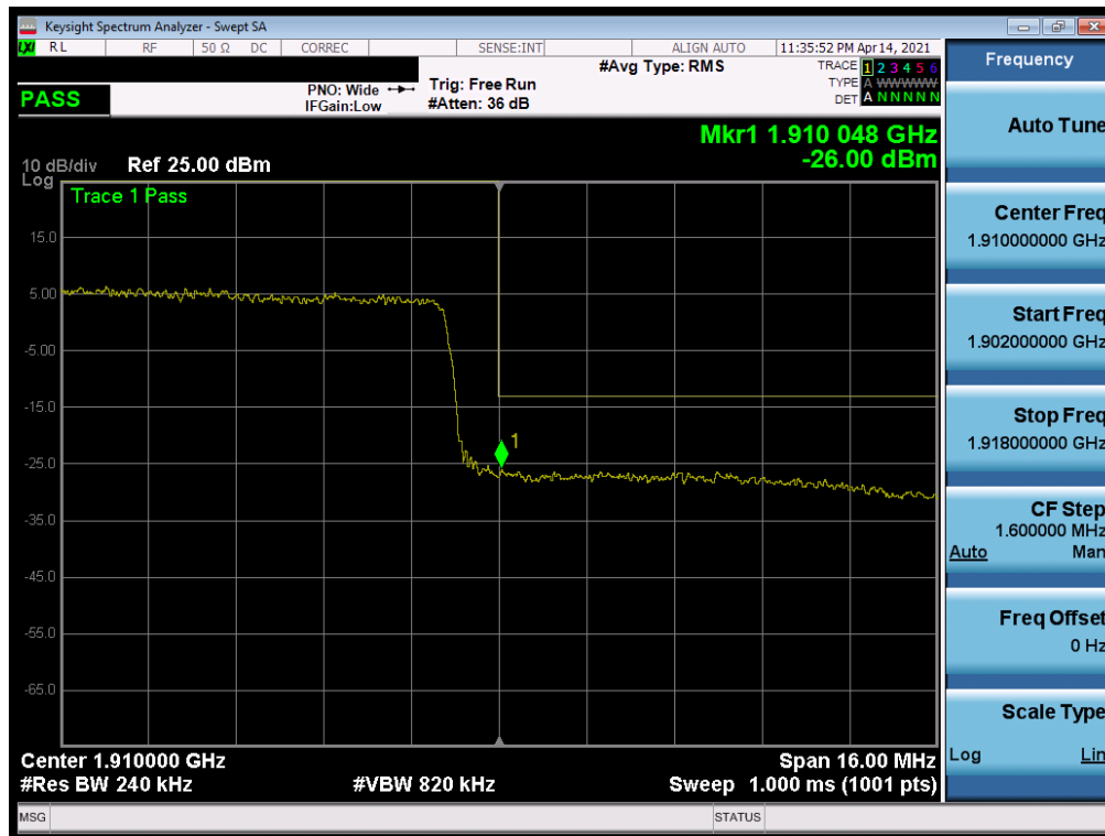
Plot 7-115. Upper Band Edge Plot (LTE Band 2 - 20MHz QPSK – Full RB)
