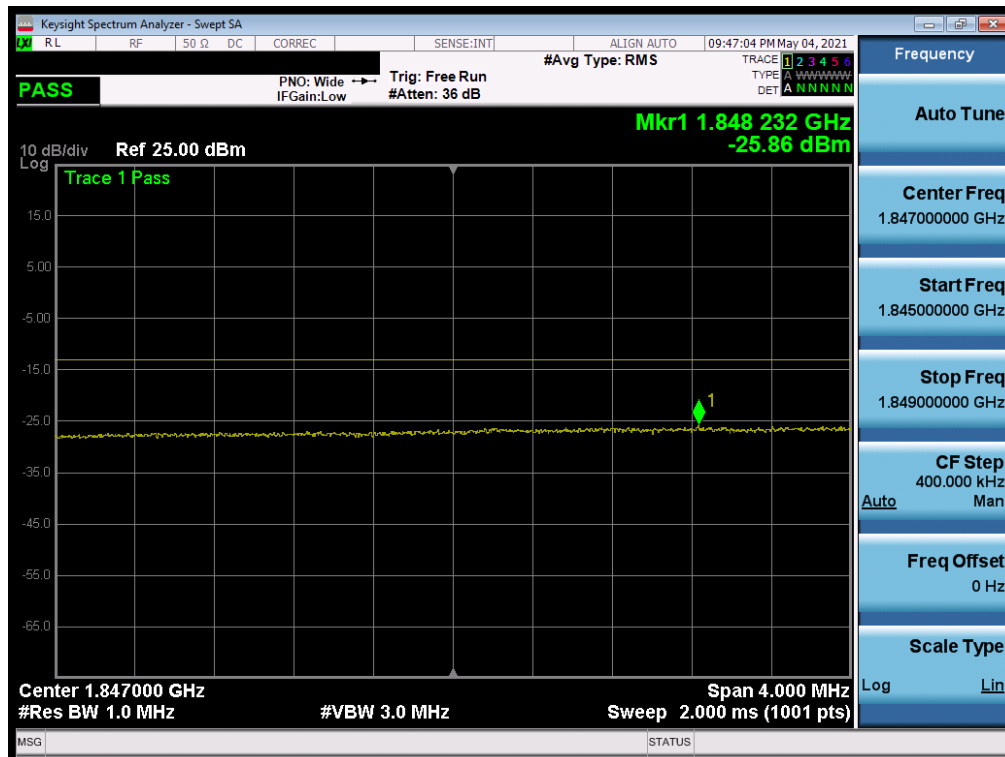
Plot 7-186. Extended Lower Band Edge Plot (NR Band n25 – 40MHz QPSK – Full RB)
