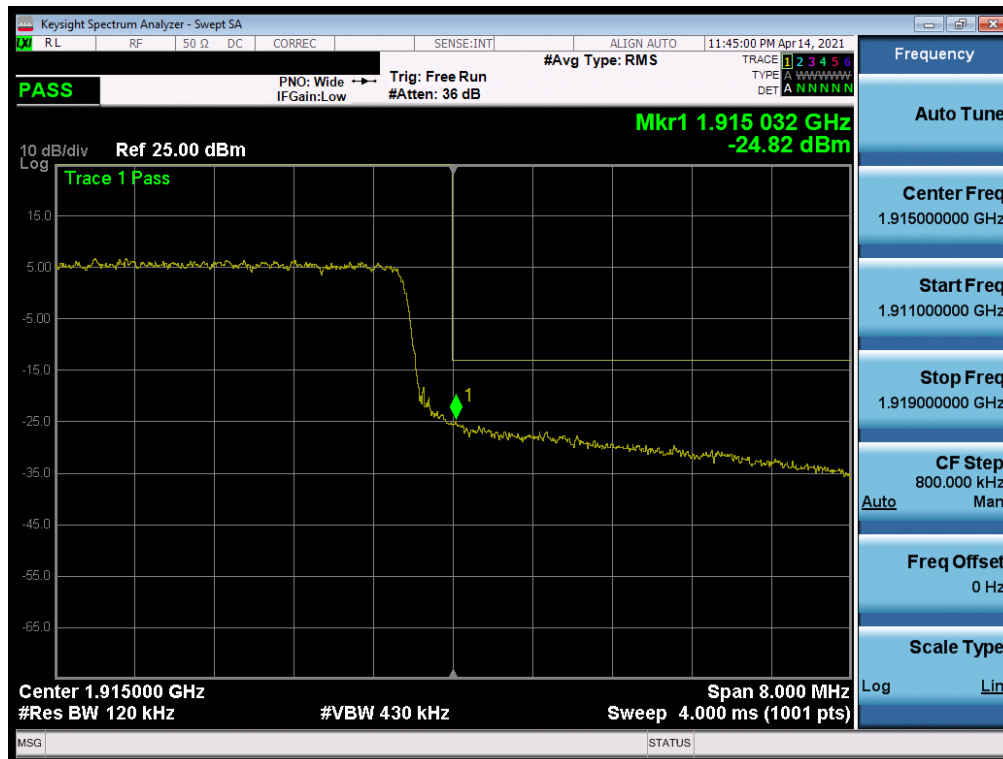
Plot 7-129. Upper Band Edge Plot (LTE Band 25 - 10MHz QPSK – Full RB)
