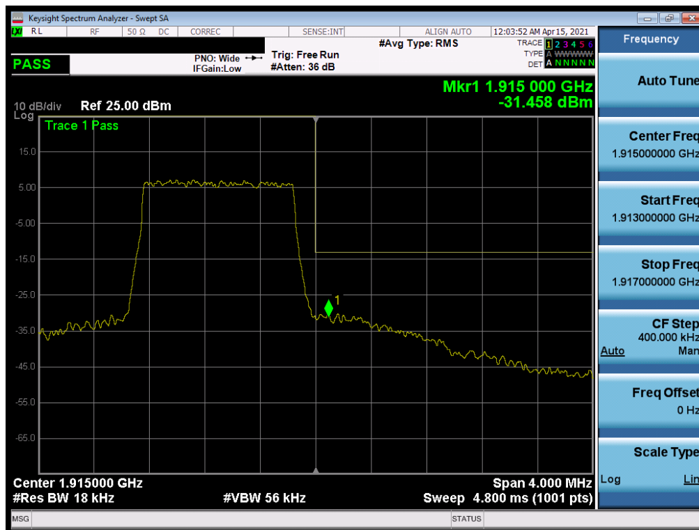
Plot 7-147. Upper Band Edge Plot (LTE Band 25 – 1.4MHz QPSK – Full RB)
