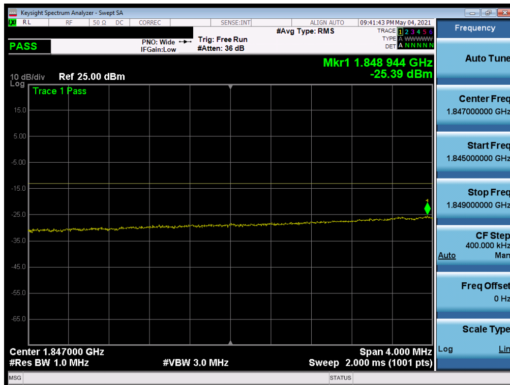
Plot 7-190. Extended Lower Band Edge Plot (NR Band n25 – 30MHz QPSK – Full RB)
