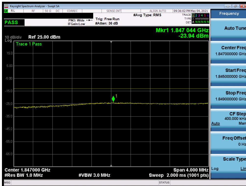
Plot 7-194. Extended Lower Band Edge Plot (NR Band n25 – 25MHz QPSK – Full RB)
