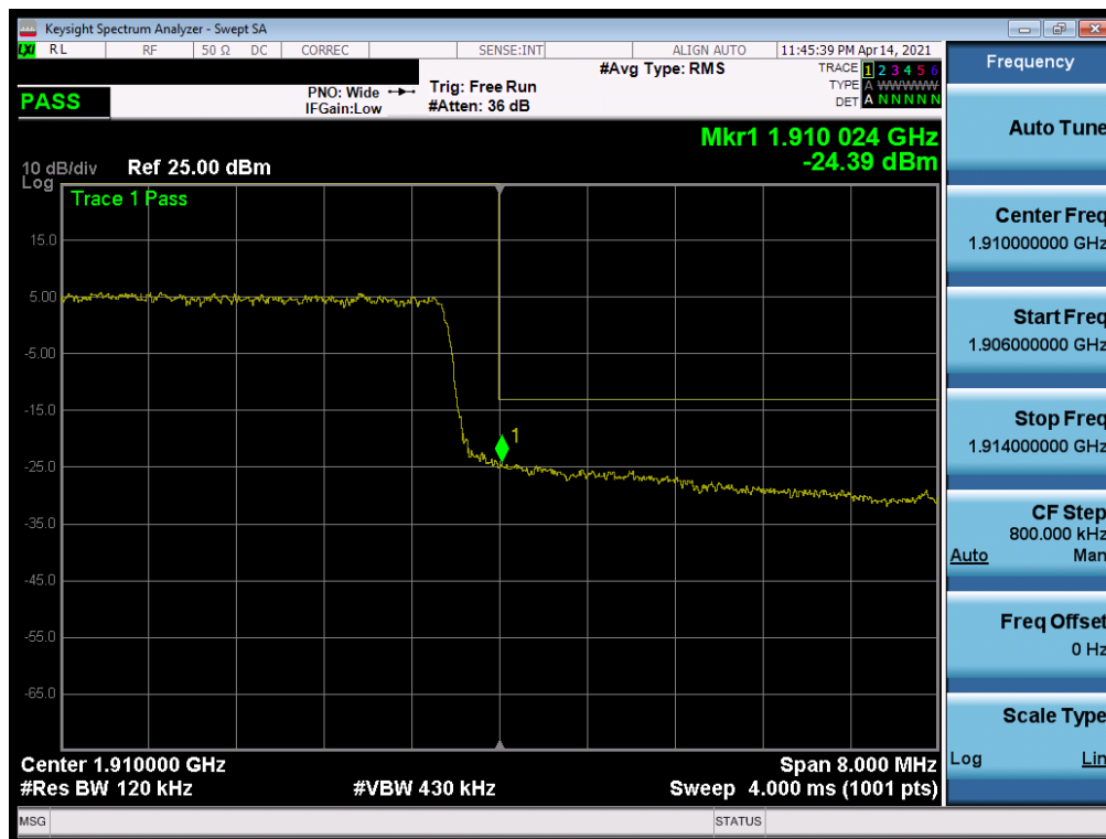
Plot 7-127. Upper Band Edge Plot (LTE Band 2 - 10MHz QPSK – Full RB)
