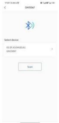
Click the scanned device to initiate a Bluetooth connection. If the connection is successful, you proceed to the next page, and the device's green light will flash to indicate a successful connection.
