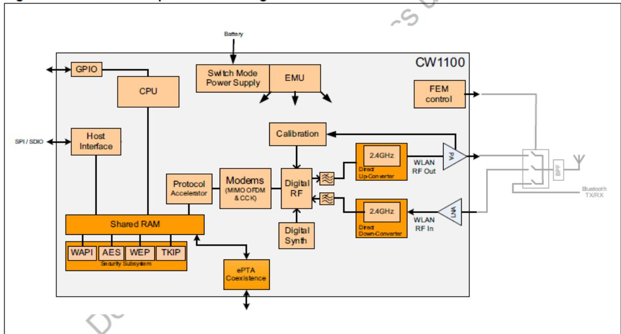
The CW1100 SoC is built on the proven success of integrating previous generation WLAN devices into cellular handsets providing the lowest power consumption, best-in-class BT/WLAN co-existence mechanism in addition to high throughput performance and better range. The CW1100 supports a comprehensive range of 802.11 standards and amendments:
