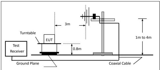
(c) For radiated emissions above 1000MHz
