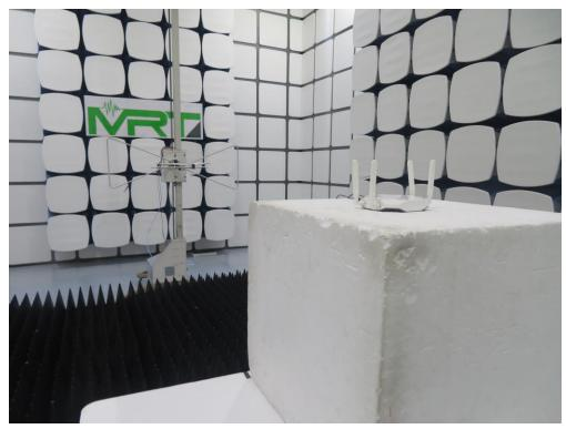
Description: Radiated Spurious Emissions Test Setup for above 1GHz\_AP321e
