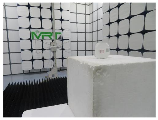
Description: Radiated Spurious Emissions Test Setup for above 1GHz\_AP321
