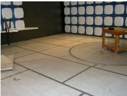
Note that Radiated Emission Test has NO ferrites. Internal modification to MMT9000 (added shielded power cable inside unit) reduced emissions sufficiently to pass Class B without ferrites. This modification was done after antenna tests, which is why ferrites appear in the setup photos for the antenna tests.
