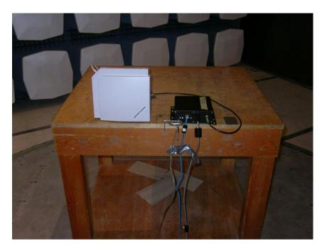
$NOTE-Modification\ to\ MMT9000\ (\ a\ shielded\ power\ cable\ internally)\ removed\ the\ need\ to\ the\ ferrites.\ See\ Radiated\ Emissions\ Test\ Setup\ above.$
