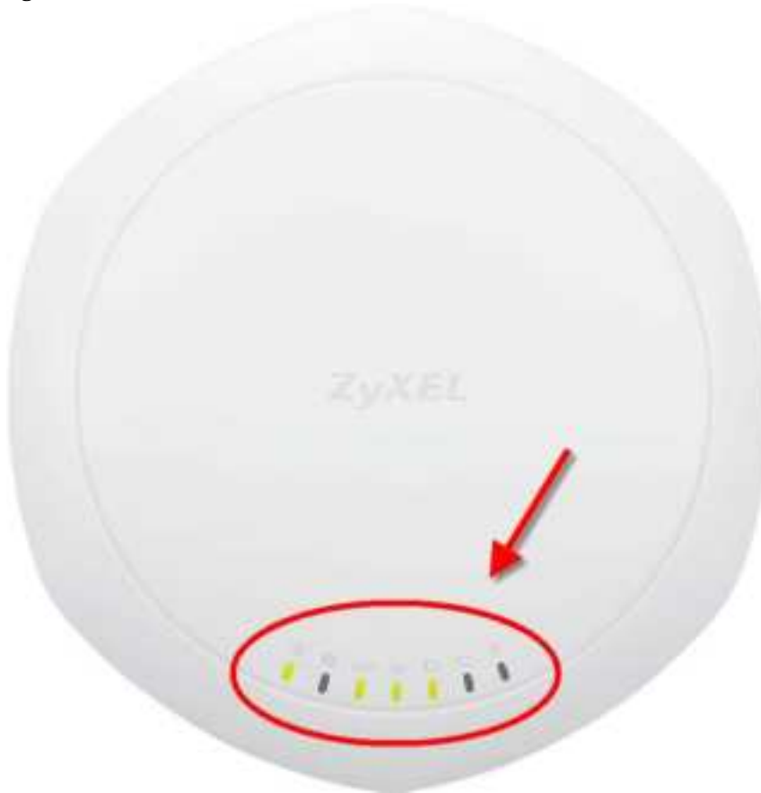
Figure 19 NWA1123-AC PRO LEDs
