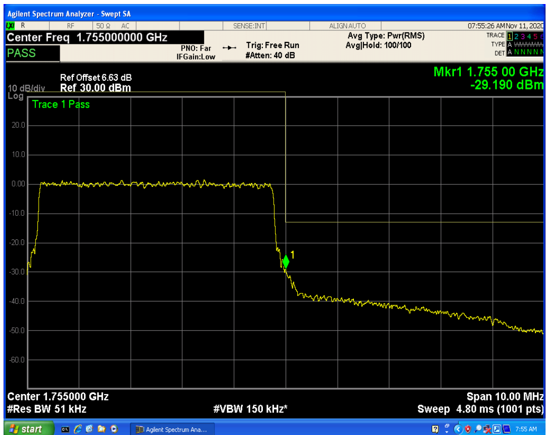
LTE Band4 QAM16 BW=5MHz Channel=20375 RB Size=1 Position=#Max
