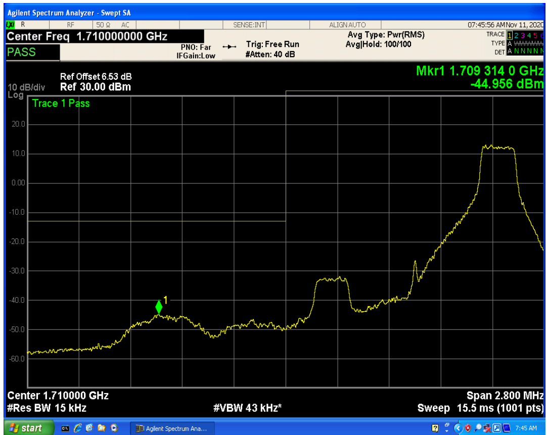
LTE Band4 QPSK BW=1.4MHz Channel=20393 RB Size=1 Position=#0
