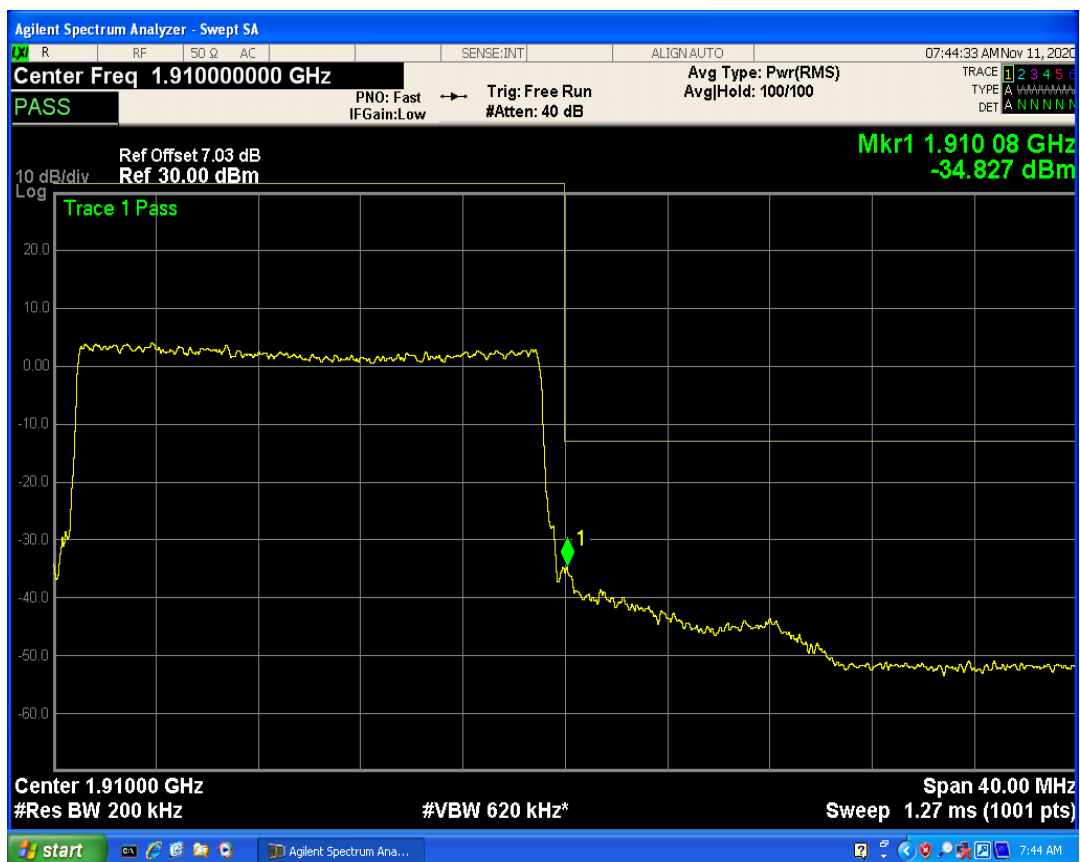
LTE Band4 QPSK BW=1.4MHz Channel=19957 RB Size=1 Position=#0
