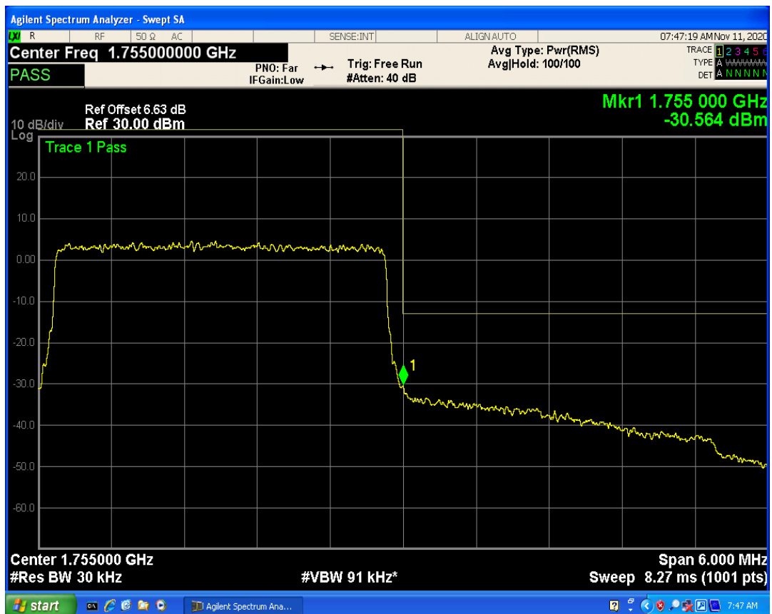
LTE Band4 QAM16 BW=3MHz Channel=20385 RB Size=1 Position=#0
