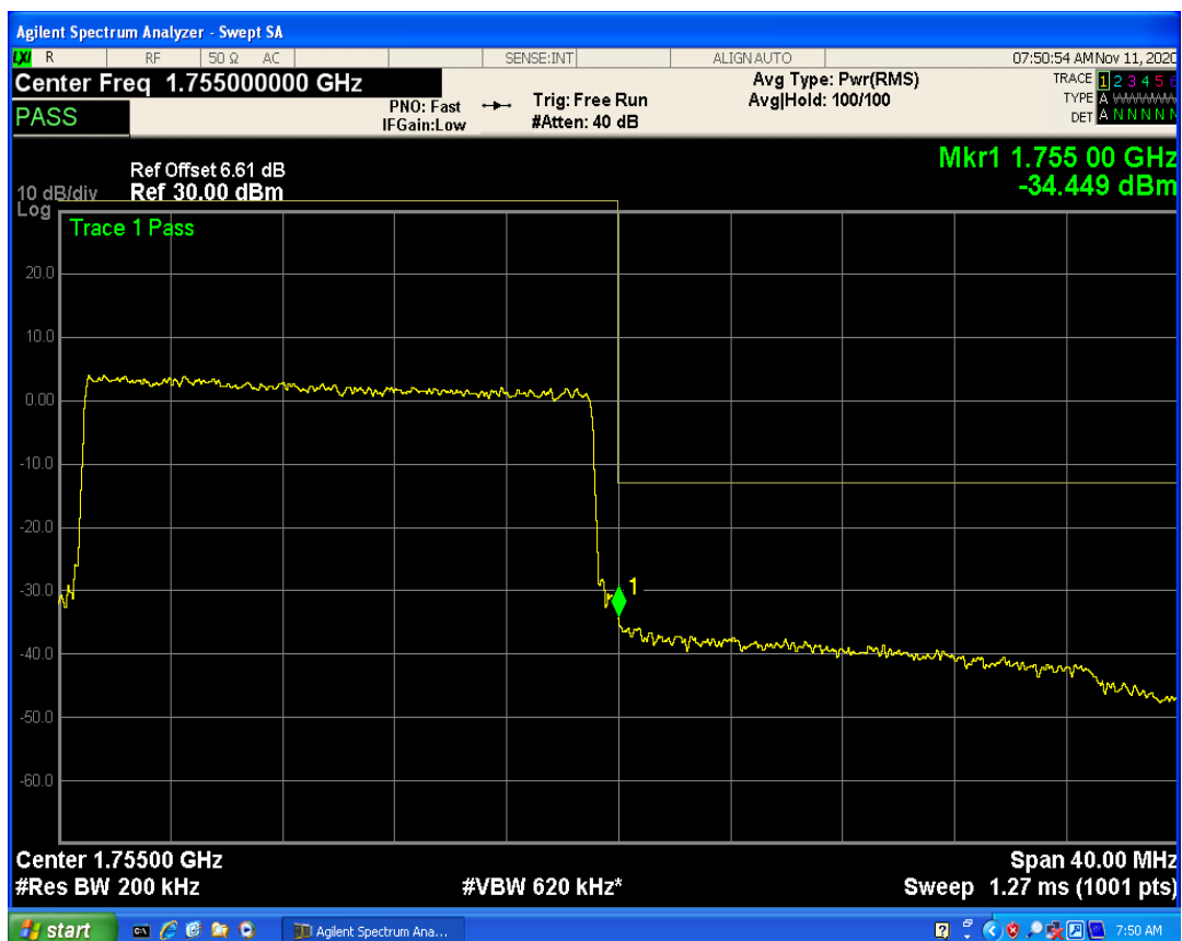
LTE Band4 QPSK BW=5MHz Channel=19975 RB Size=1 Position=#0
