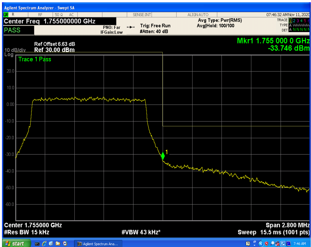
LTE Band4 QPSK BW=3MHz Channel=19965 RB Size=1 Position=#0
