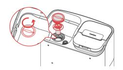
2 Remove the Waste Filter inside, and rinse it under a tap.
