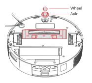
**2** Rinse the wheel and axle to remove hair or dirt. Dry it and reattach the wheel, pressing it firmly into place.
