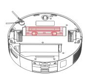
**2** Remove the Anti-Tangle Rubber Brush, pull out the bearings at both ends, and clean any hair or dirt wrapped around the brush. You can use the provided small cleaning tool for this.
