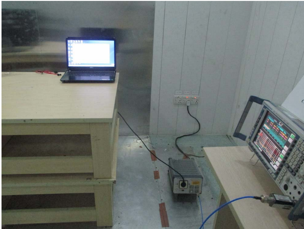
FCC RADIATED EMISSION TEST SETUP
