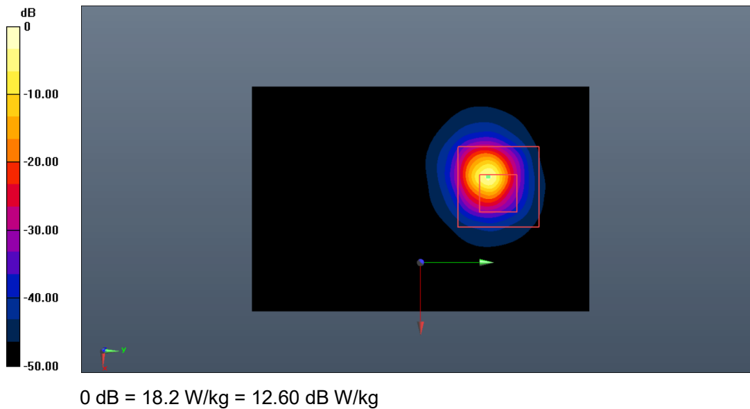
Fig.B.8. Validation 5250MHz 100mW
