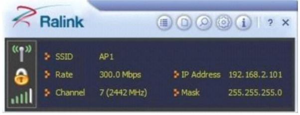
TheRalinkwirelessutilitystartsincompactmodeasshownabove, provides profilemanagement, the available networks listing, astatistical counterdisplay, Wi-Fimultimedia (WMM), protected Wi-Fi setup, Ciscocompatible extensions (CCX), callad mission control (CAC), radiocontrols, Ralink
