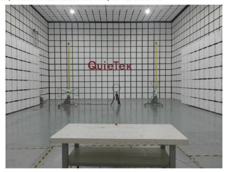
Description: Radiated Emission Test Setup for 30MHz~1GHz
