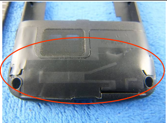
GSM/PCS/UMTS-FDD Antenna View
