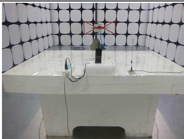
Radiated Spurious Emissions Test Setup Below 1GHz
