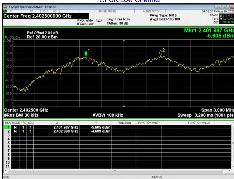
Test plots GFSK Low Channel
