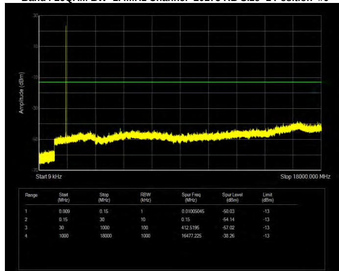
Band4 16QAM BW=1.4MHz Channel=20393 RB Size=1 Position=#0
