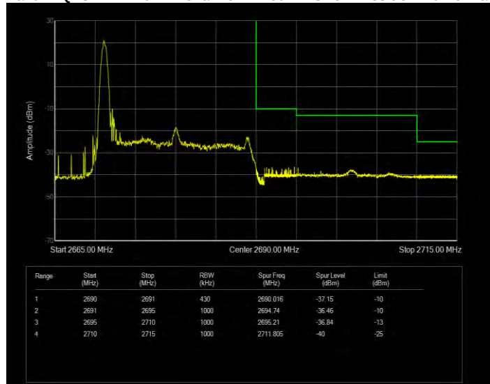
Band41 QPSK BW=20MHz Channel=41490 RB Size=1 Position=#Max Extended
