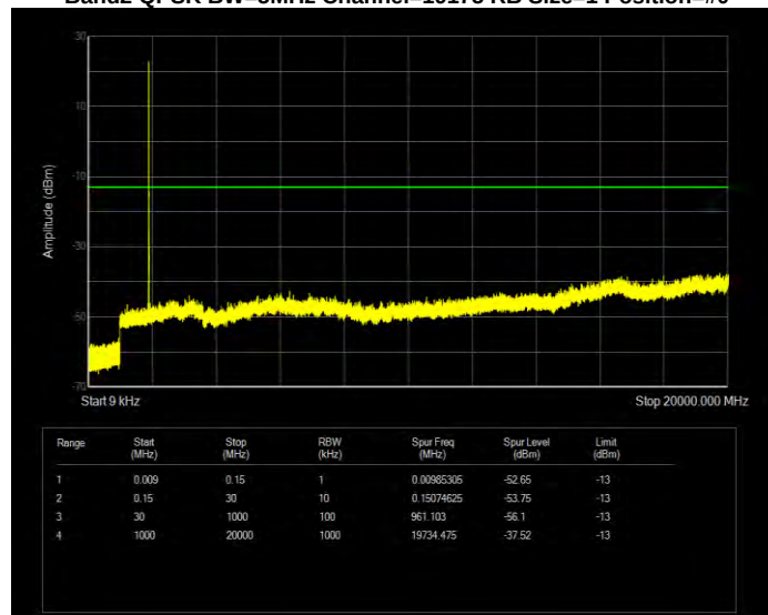
Band4 16QAM BW=1.4MHz Channel=19957 RB Size=1 Position=#0
