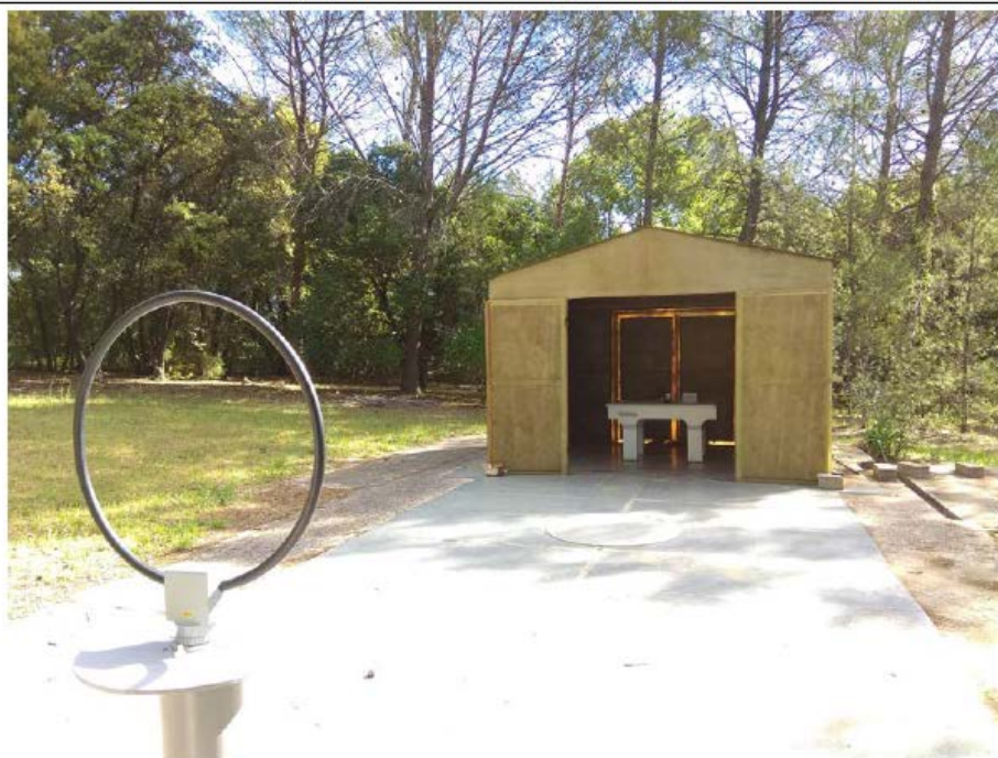
TEST SETUP PHOTO(S) RADIATED EMISSION(F<30MHZ, FINAL MEASUREMENT)
