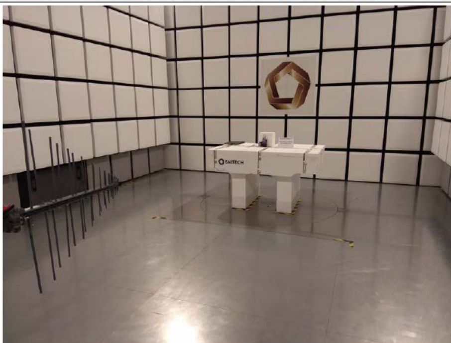
TEST SETUP PHOTO(S) RADIATED EMISSIONS (200MHZ-1GHZ)
