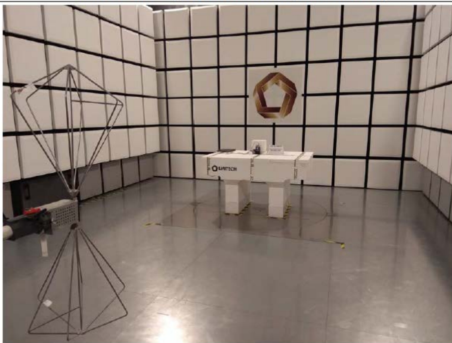
TEST SETUP PHOTO(S) RADIATED EMISSIONS (30MHZ-200MHZ)
