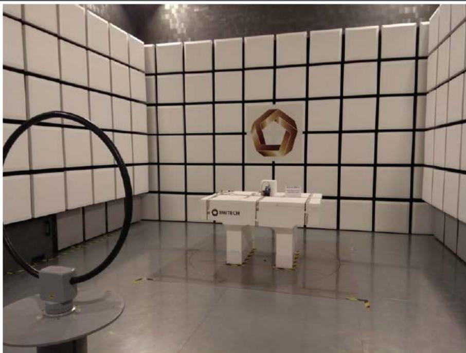
TEST SETUP PHOTO(S) RADIATED EMISSION(F<30MHZ, PRE MEASUREMENT)
