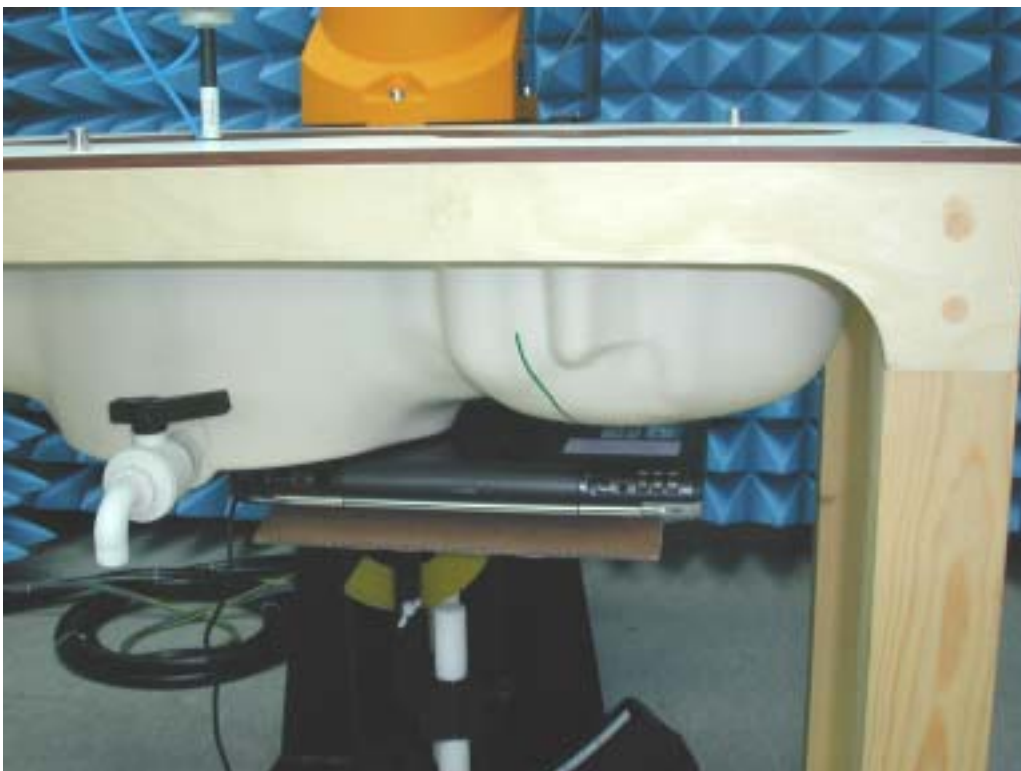
Fig.4 Photograph of the top cover parallel and at a distance of 1.5 cm from the base of the phantom
