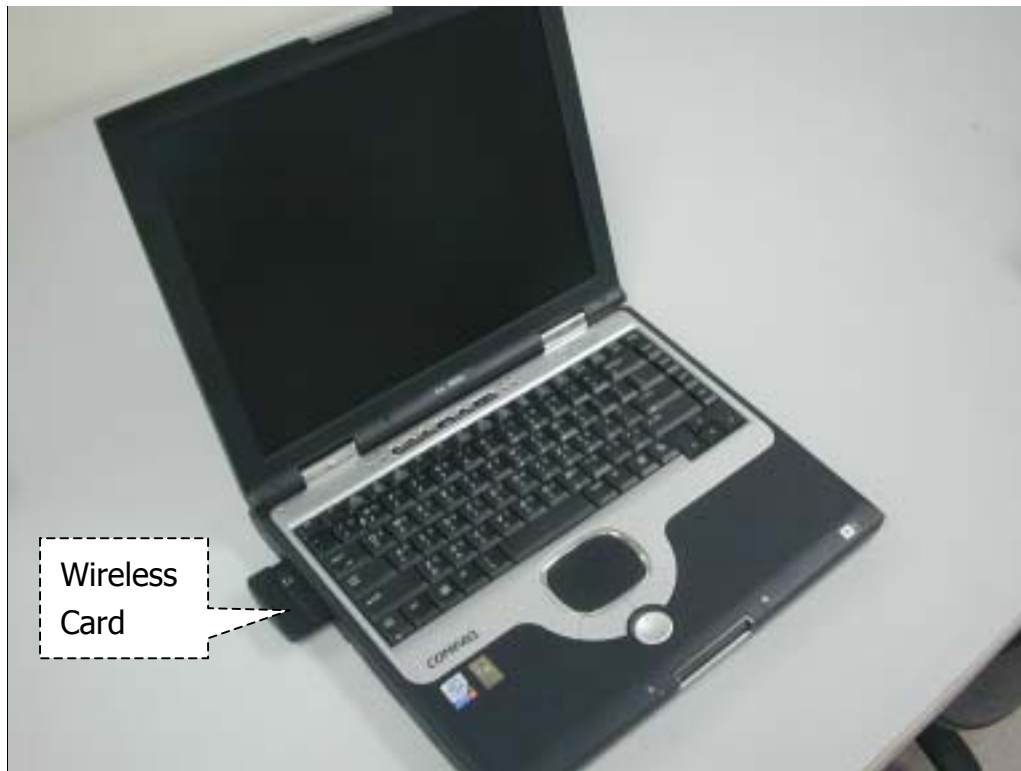
Fig.11 with COMPAQ N800 Host Laptop PC PCMCIA slot
