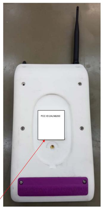
Label with **FCC ID:2ALN6200** will be located at the rear side of the logger. The statement according to FCC part 15 §15.19(a)(3) is placed in User's Manual, page 3 (Application exhibit User\_manual\_29352).
