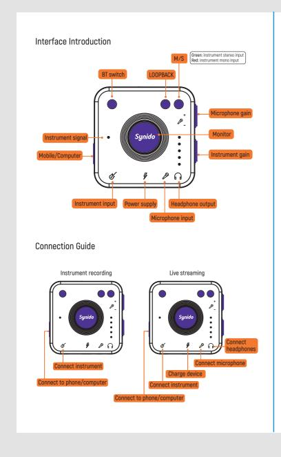
The Synido LiveDock A20 is a portable instrument recording audio interface with a dual-core chip and a high-performance 32-bit DSP core. It features independent high-performance AD/DA conversion supporting 24-bit, 96 kHz audio sampling.
