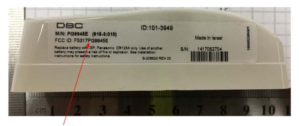
Label with **FCC ID:F5317PG9945E** is located at the side panel. The statement according to FCC part 15 §15.19(a)(3) is placed in User's Guide, page 1 (Application exhibit User\_manual\_29734).
