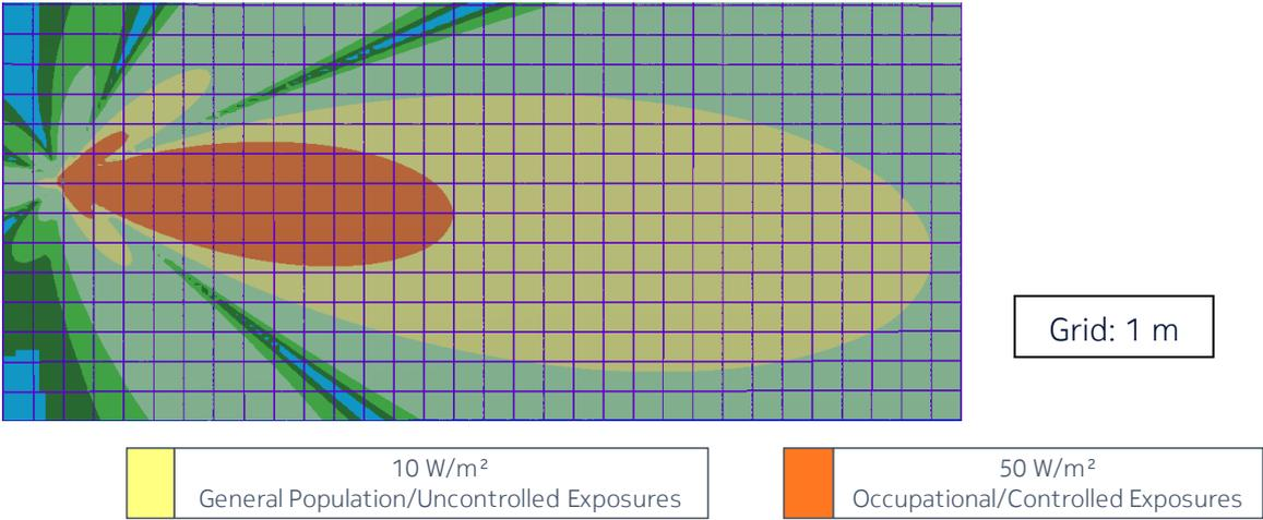
Figure 4 – Side view of the power density for the time-averaged maximum transmitted power of 339 W (EU/ICNIRP, Australia/NZ and US/related)
