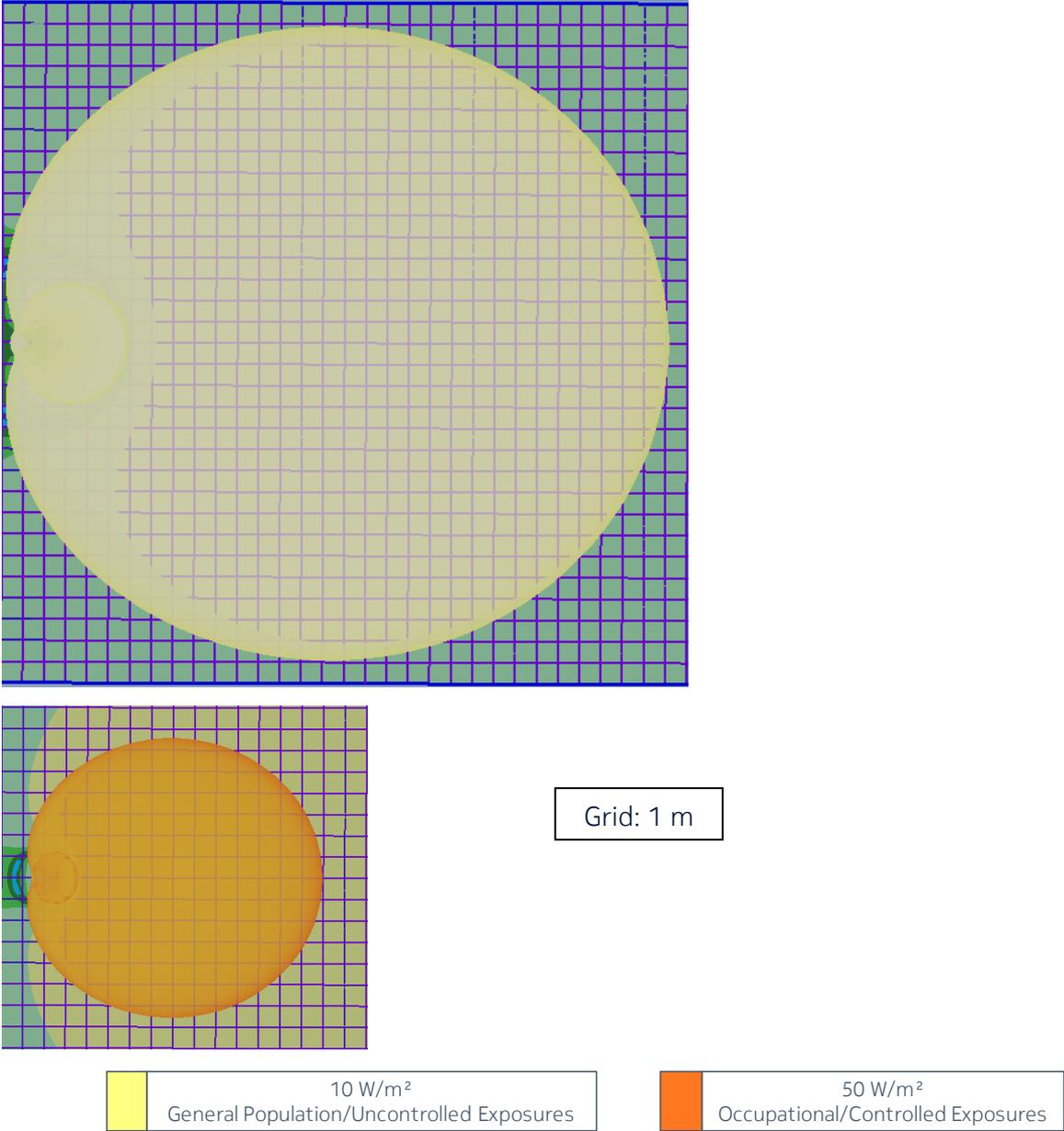
Figure 2 – Top view of the power density for the time-averaged maximum transmitted power of 339 W (EU/ICNIRP, Australia/NZ and US/related)
