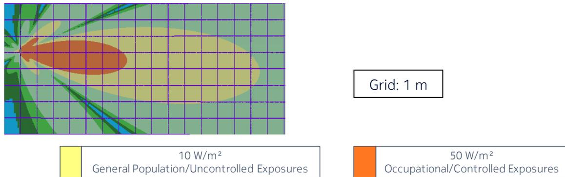
Figure 5 – Side view of the power density for the time-averaged actual maximum transmitted power of 85 W (EU/ICNIRP, Australia/NZ and US/related)
