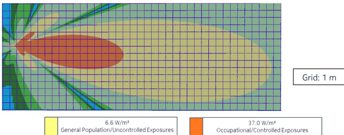
Figure 8 – Side view of the power density for the time-averaged maximum transmitted power of 339 W (Canada)
