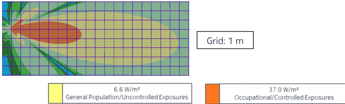
Figure 9 – Side view of the power density for the time-averaged actual maximum transmitted power of 85 W (Canada)
