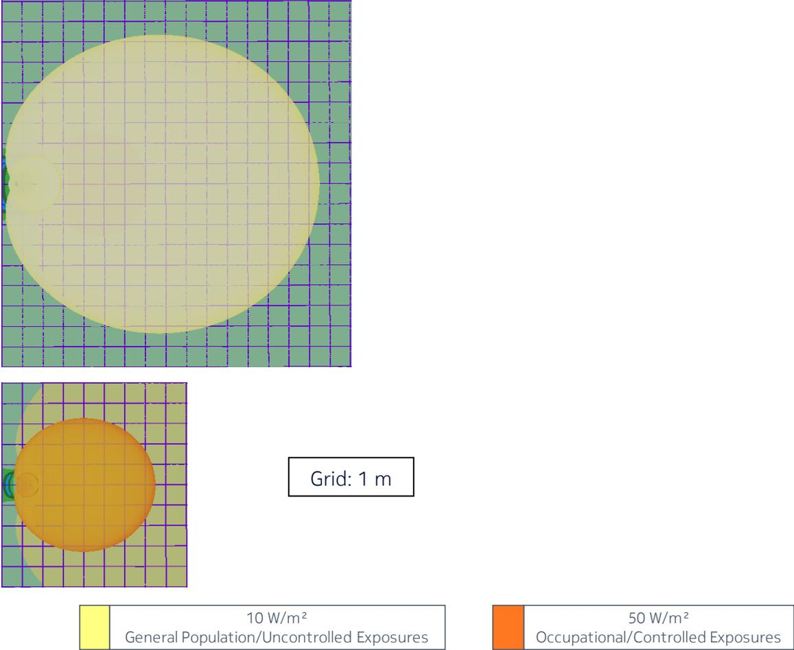
Figure 3 – Top view of the power density for the time-averaged actual maximum transmitted power of 85 W (EU/ICNIRP, Australia/NZ and US/related)
