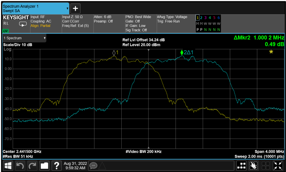
Figure 48 - \pi/4 DQPSK - 2441 MHz (CH39)
