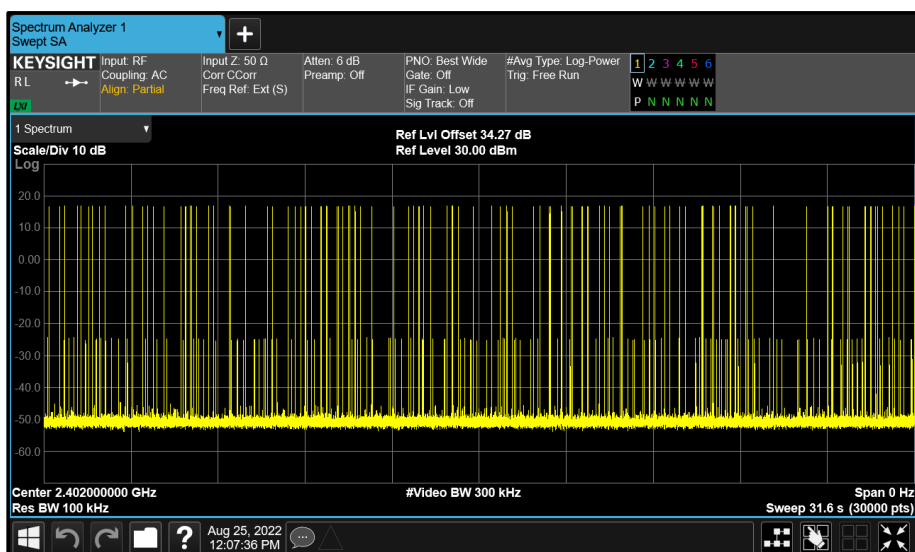
Figure 27 - \pi/4 DQPSK - 2402 MHz Accumulated Transmit Time
