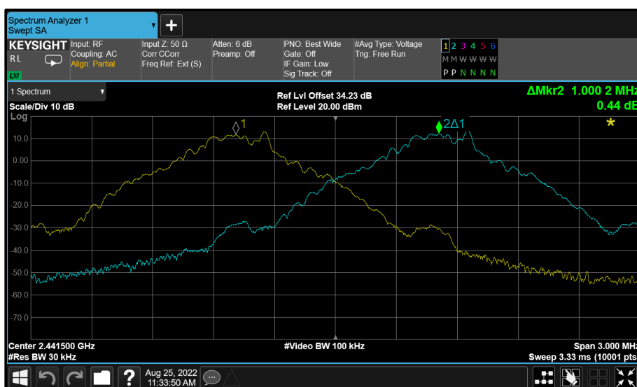
Figure 45 - GFSK - 2441 MHz (CH39)
