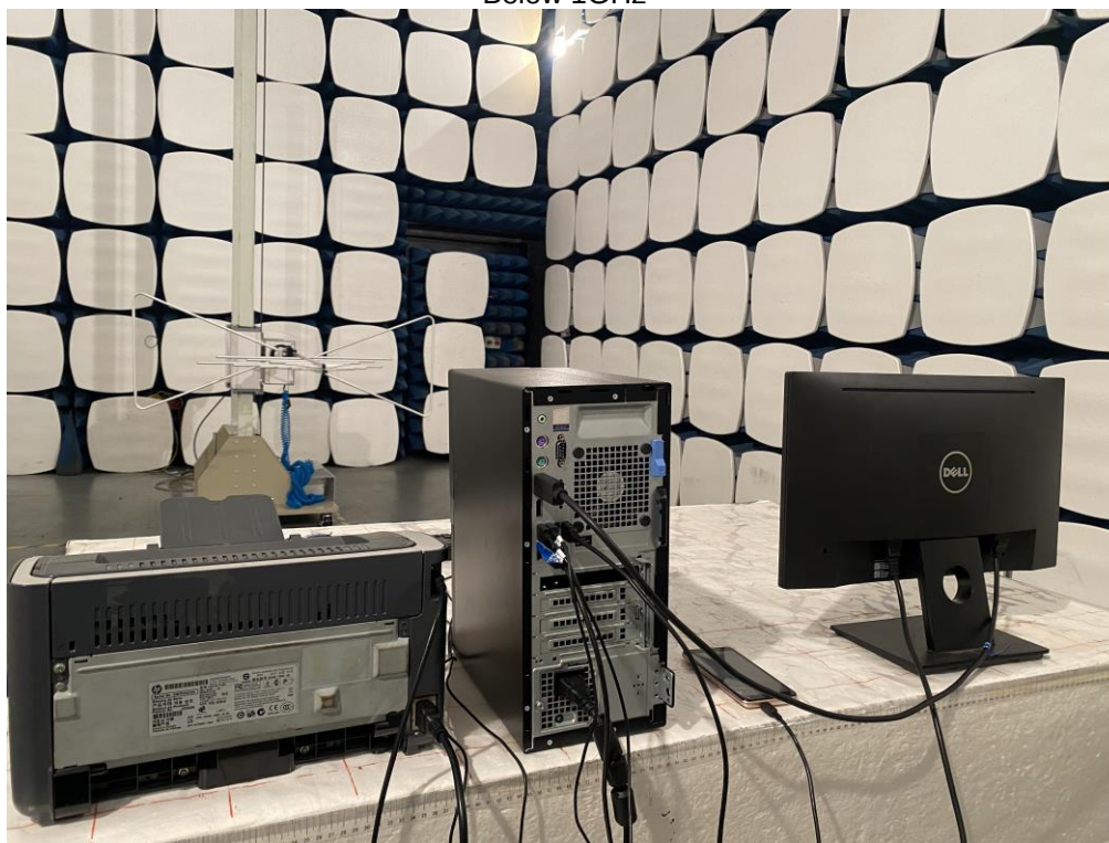
Radiated Emission Below 1GHz
