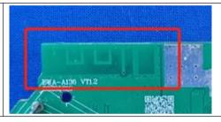
The antenna is PCB antenna.
