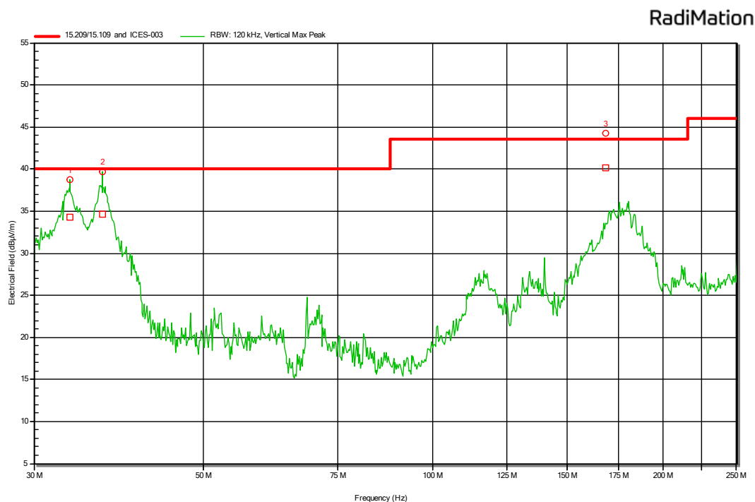
Plot 1f: radiated emissions of the EUT, Antenna vertical, in the range 30 – 250 MHz (pre-scan peak values shown) High channel
