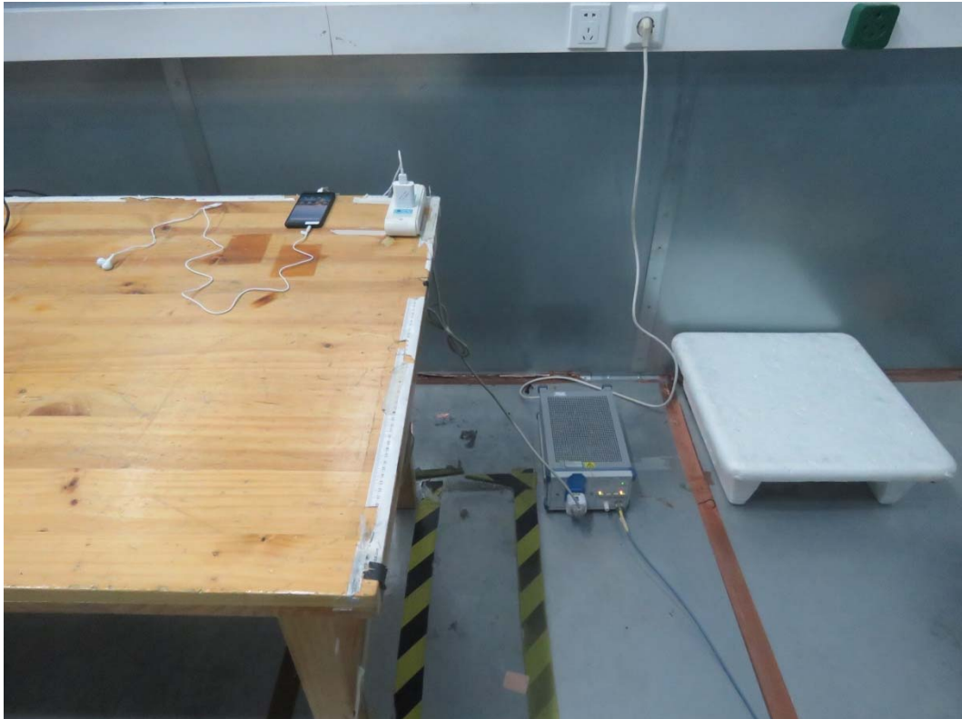
Picture 2 Conducted Emission Test Setup
