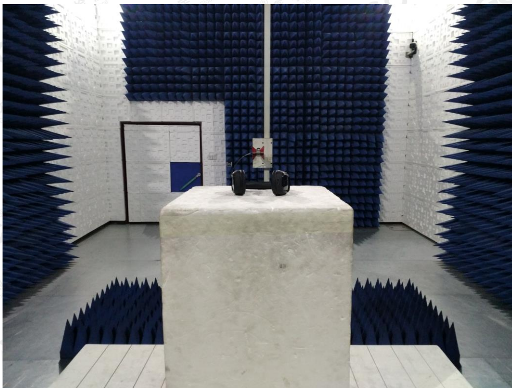
RADIATED EMISSION TEST SETUP ABOVE 1GHZ
