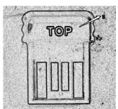
Conclusion: Based on the above description of area A to B, we conclude that the device is unquestionably too small for enabling the FCC certification No. to be printed onto any surface. We therefore request to move the FCC certification No. to the user's manual.
