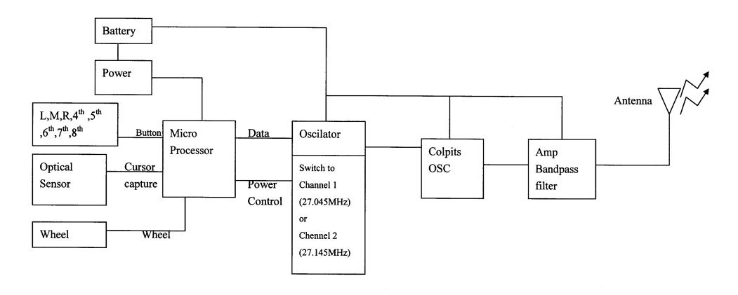
Model: RFSWOP-80 Wireless Radio Wheel Mouse (Transmitter)
