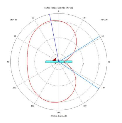
Frequency = 2.45 GHz Main lobe magnitude = 0.173 dBi Main lobe direction = 11.0 deg. Angular width (3 dB) = 294.0 deg.
