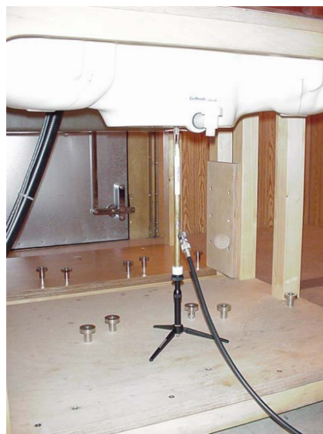
2450MHz Dipole Setup
