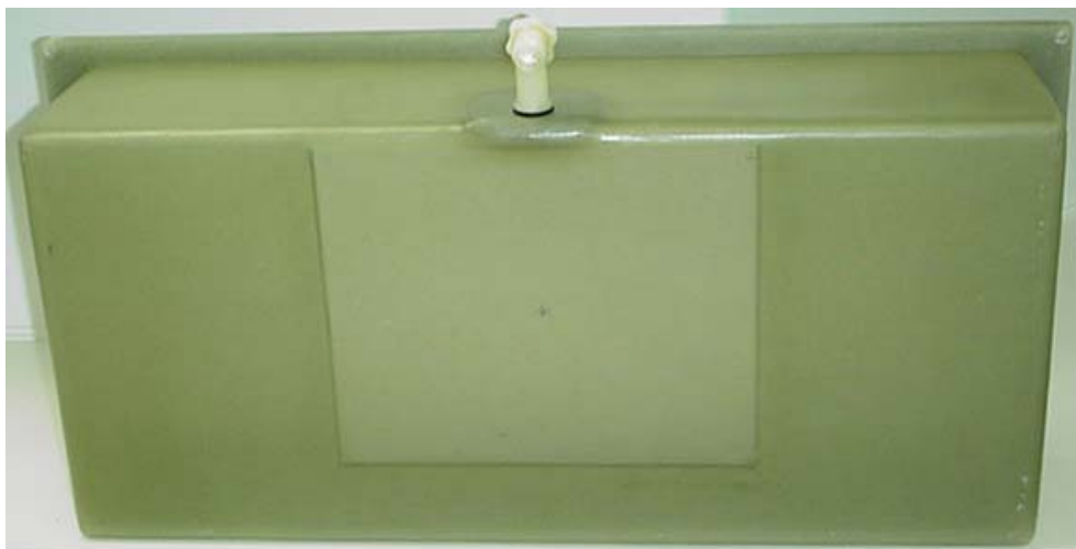
Fiberglass Planar Phantom - Bottom View
