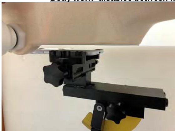
Fig.7 EUT Front side to flat phantom
