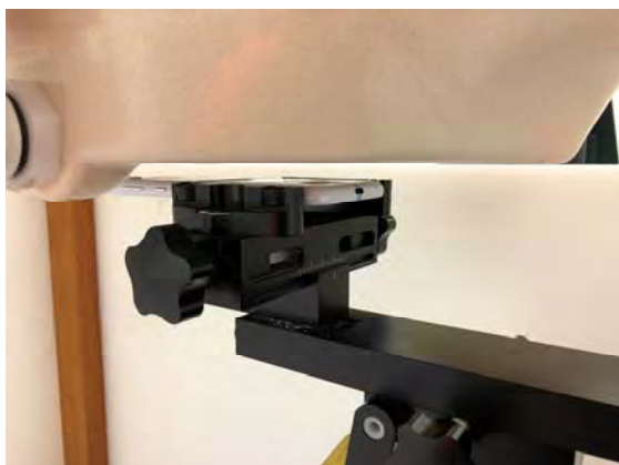
Fig.10 EUT Back side to flat phantom
