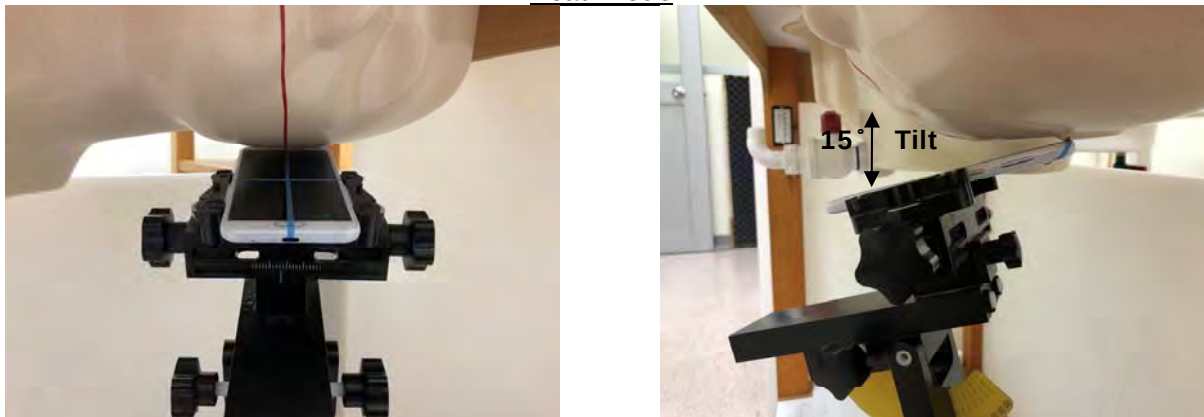
Fig.6 Left Head Section / Ear-Tilt Position(15°)
