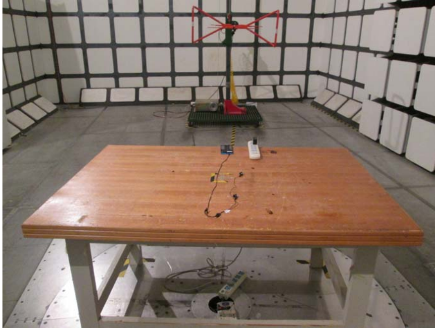
Radiated Emissions – Front View (30-1000 MHz)
