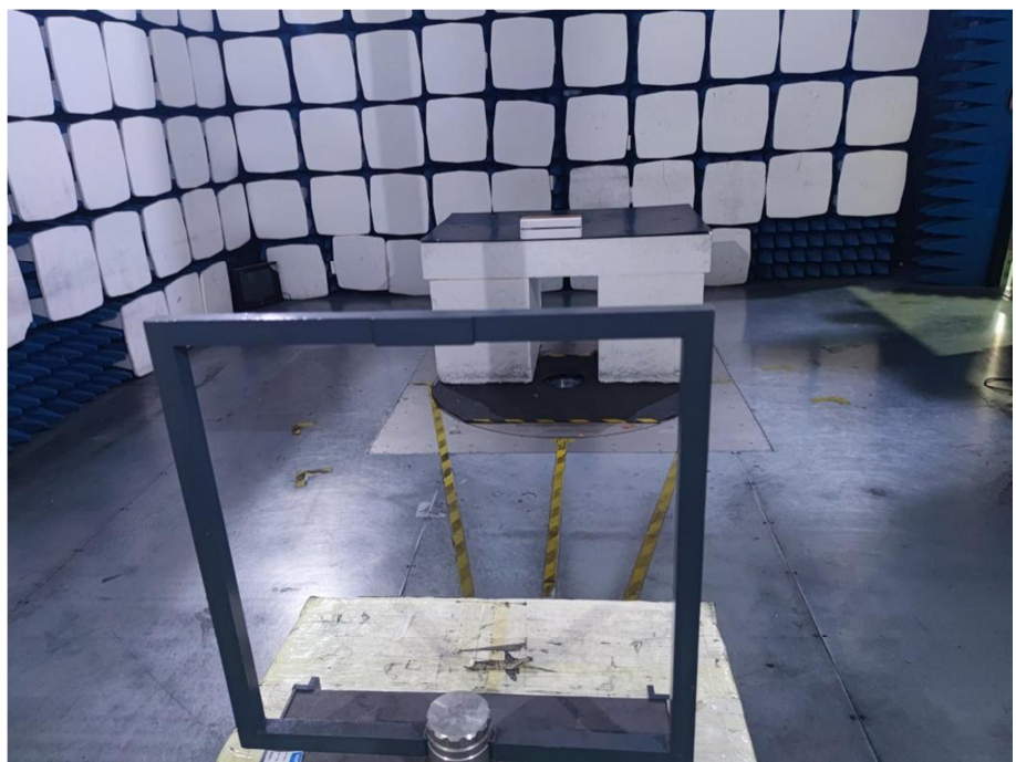
Radiation Emission Test Setup (Below 30MHz)
