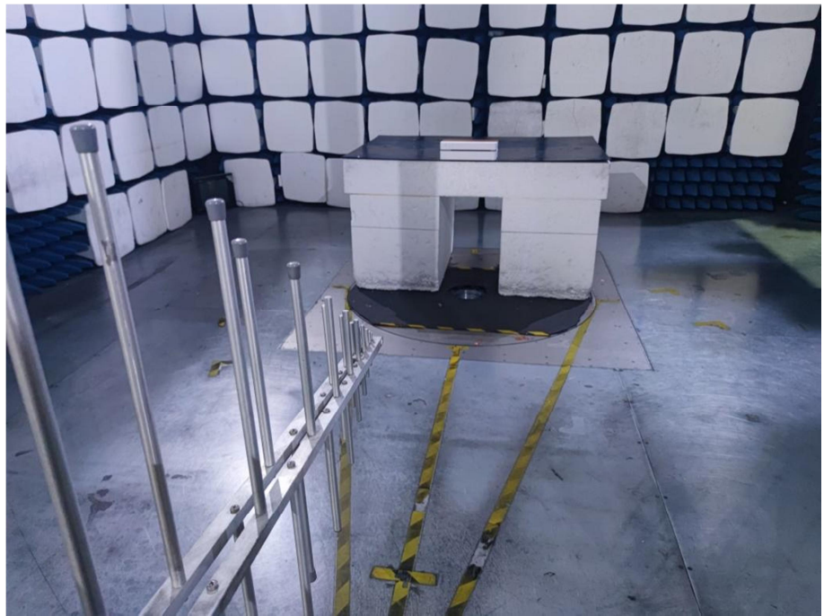
Radiation Emission Test Setup (30MHz to 1GHz)
